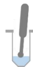
6. Wash crystal crusher in cooled reservoir solution in seed bead tube to collect seeds from crystal crusher
