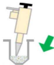
9. Transfer the mixture back to the Seed Bead tube. Repeat the process until no crystals are visible in the drop.
