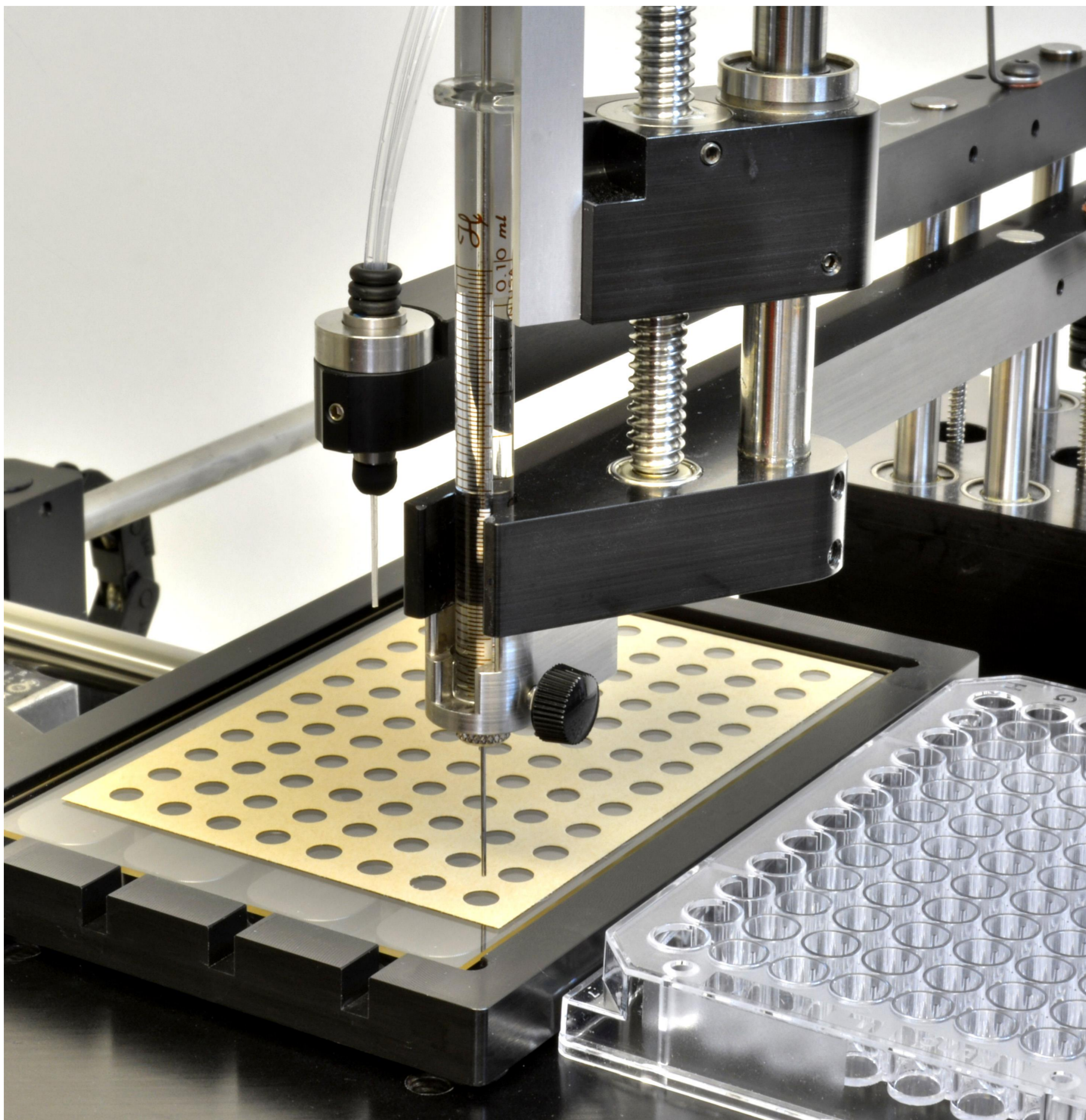
Dispensing LCP to glass sandwich plates
